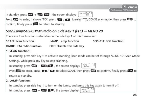
Press went to enter, press / to select LAMP, then press to confirm, finally press to return to standby.
